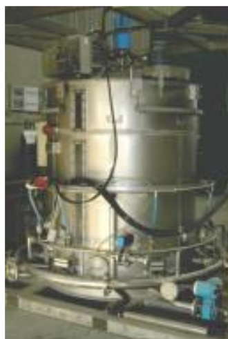
Slika 3 Dissolved Air Flotation System (DAF)
